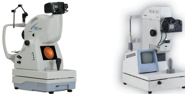
Fig. 3. Two retinal image cameras. The retinal image is acquired by taking an instant photograph.
